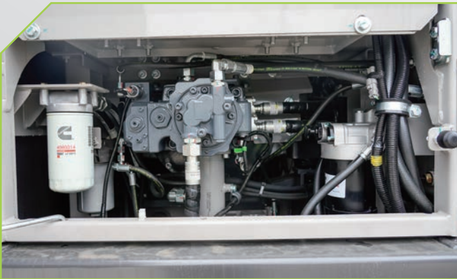
Engine fuel filters, oil filter, air cleaner, hydraulic oil pilot filter and A/C filter are easily accessible at ground level, achieving "one-stop" maintenance on the ground.
