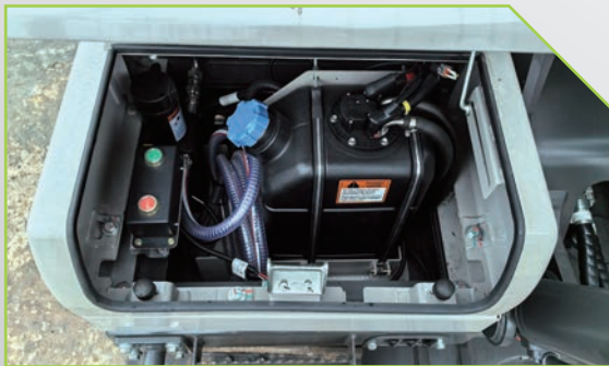
It's easy to fill the DEF tank, which is placed in the toolbox.
